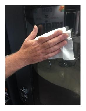
3. Take the SAFE TOUCH film and apply it with the backing to the front of the screen, ensuring the film is aligned to the top and sides of the glass screen. Fix it in place with masking tape. TIP – Peel the ends of the masking tape up to ease removal later
