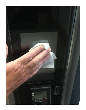
3. Take the SAFE TOUCH film and peel back the rear release layer by approx. 15mm and fold it over to provide a datum edge to align to the top of the touchscreen.
