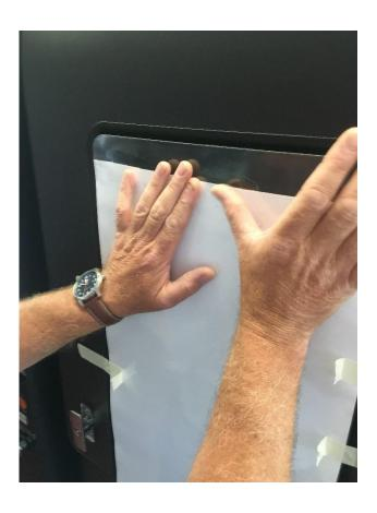
6. Remove the masking tapes to allow you to lift the SAFE TOUCH film. The larger film for COTI & CALI is best applied wet with a water and washing up liquid solution
