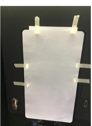
4. With the SAFE TOUCH film secured with masking tape, peel back to release layer by approx. 15mm to provide a datum edge to align to the top of the touchscreen. TIP – it may be easier to cut the release layer than folding it.
