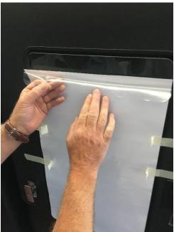
5. Fit the top edge of the SAFE TOUCH film to the top of the touch screen and work it down.
