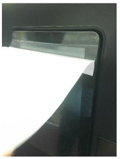
9. Using the graphic squeegee applicator apply the SAFE TOUCH screen top edge and then work down the touchscreen as you remove the release layer. Take care to apply the screen slowly removing any air bubbles as you go. Work all the way to the bottom of the screen, ensuring all edges are worked down.
