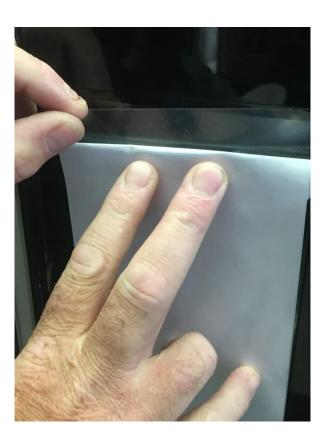
4. Fit the top edge of the SAFE TOUCH film to the top of the touch screen.
