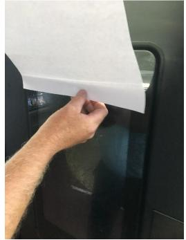
7. With the SAFE TOUCH film lifted up, spray the glass with your water and washing up liquid solution. Note; you only need a very small amount washing up liquid.
